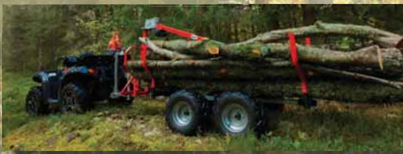
Dimensiones: Ancho 1200mm x Alto 1100mm x Largo ajustable 2800mm - 4000mm
